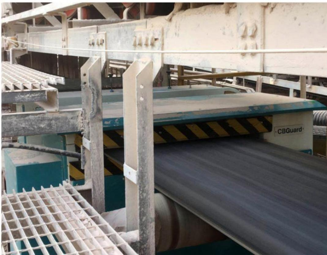
*The CBGuard Life Extender provides all-in-one radiographic conveyor belt monitoring, continuous real-time analysis and reporting, and detection and live marking of all defects/damages associated with splice failures, among other things, the company says, with “every cubic millimetre of the conveyor belt analysed”*
