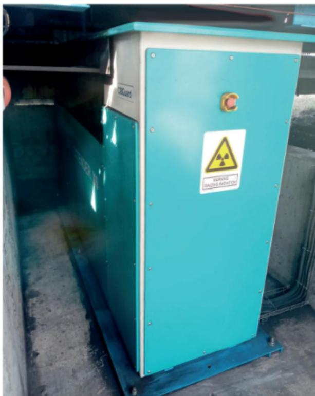
Figure 2. A CBGuard in a coal handling conveyor.
